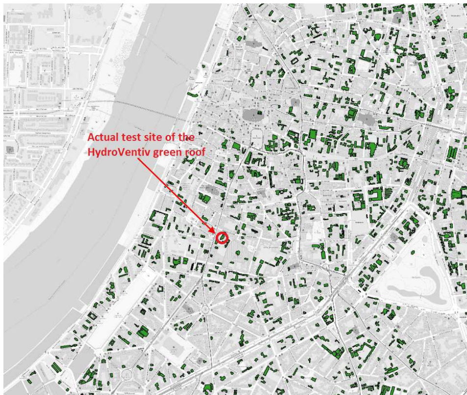
Figure 7.25. Potential green roof map for Antwerp creating through the newly developed algorithm, indicating where green roofs can be installed.
