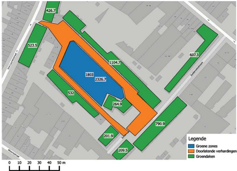
Figure 7.26. Implementation of a cluster of innovations: green zones (shown in blue), permeable pavement (orange) and green roofs (green). These innovations can be simulated individually or simultaneously in SCAN.
