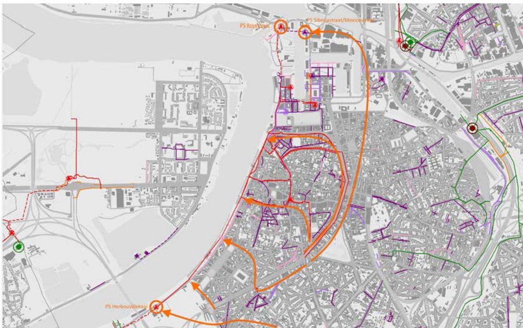
Figure 7.9: Schematic overview of the drainage directions and main flow pipes in Antwerp (source: Riolink; sewer manager of the city of Antwerp).
