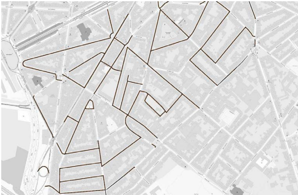
Figure 7.27. Identified roads in the flood prone Brederode district to implement permeable pavement.
