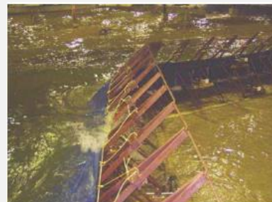
Figure 7: Example testing of a 'porta dam' using to the USACE guidelines for testing (Wibowo & Ward 2016)
