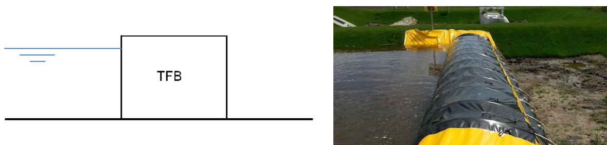
Figure 5-3 Schematic cross section of a theoretical Temporary Flood Barrier (TFB) (left) and a picture of a TFB (right) (source: www.tubebarrier.com )
